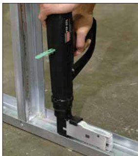
Rotating magazine allows for installation flexibility.
