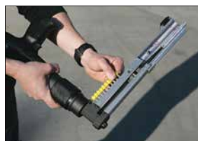
Collated pins for fully automatic fastening and quick loading.
