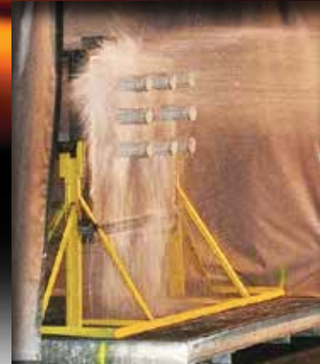
Hose stream test
