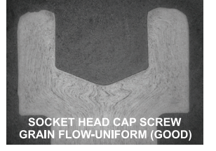
SOCKET HEAD CAP SCREW GRAIN FLOW-UNIFORM (GOOD)
