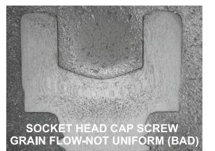
SOCKET HEAD CAP SCREW GRAIN FLOW-NOT UNIFORM (BAD)
